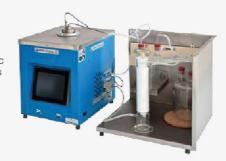
Test Method: PP = ASTM D6749, ASTM D97, ISO 3016 Sample Required: 150ml
